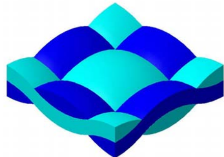
Fig. 3 Tow model of plain weave
