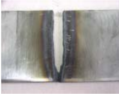
Fig 9. Stainless steel materials by cutting hybrid combustion cutter
