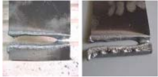
Fig 8. Normal steel materials by cutting hybrid combustion cutter
