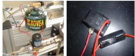
Fig 5. hybrid cutter's Ignition equipment
