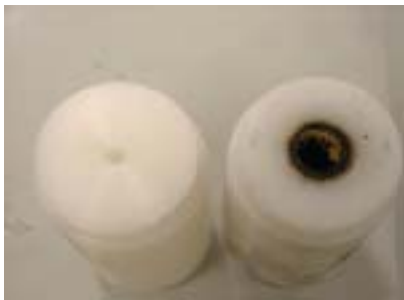
Fig 10. Solid Fuel(PE) shape before and after combustion
