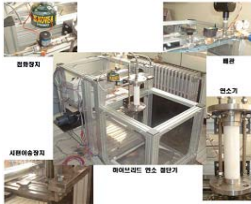
Fig 3 Lab-scale hybrid rocket cutter experiment
