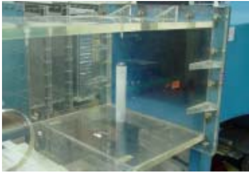
(a) Single circular tube without vortex generator
