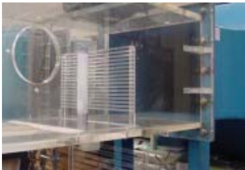
(b) Single circular tube with vortex generator
