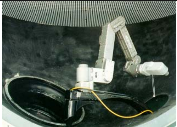
Fig. 7 The appearance of nozzle dam installation/removal robotic system.
