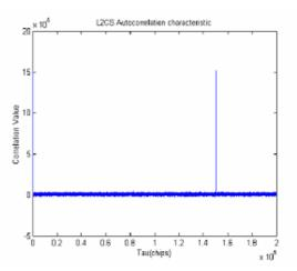
Fig 7. Autocorrelation characteristics of L2CS code
