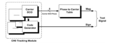
Fig 14. Test Signal Generator.
