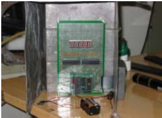
Fig. 2 The testing controller board surrounded by plumbum (Pb) blocks at the Cyclotron accelerator
