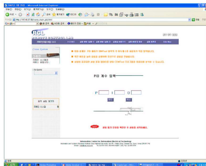
Fig. 5. Page with three boxes for coefficients of PID controls
