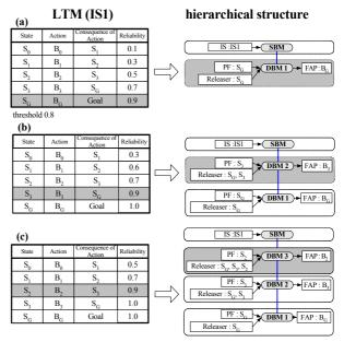
Fig. 7. An example of interaction between LTM and hierarchical structure.
