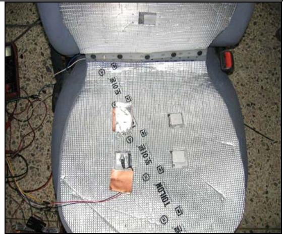
Fig. 6 the appearance developed hot and cool temperature control system in the car-seat
