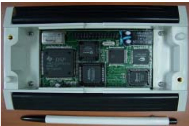
Fig. 4 Master Controller based on LonWorks network
