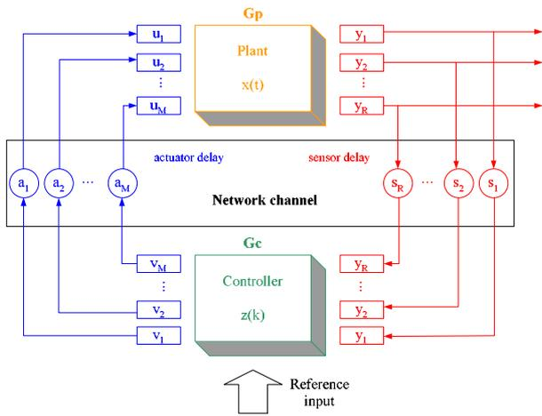
Fig. 2 The block diagram of an NCS
