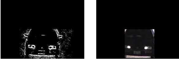
(b) A result of difference (c) An extraction result Fig. 1. Car domain extraction
