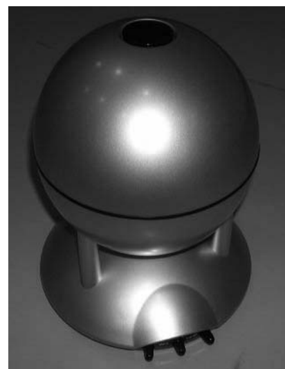
Fig.2 Photography of non-directivity speaker SEP-01, by Sugiyama Electron Co. Ltd. (in Japan).
