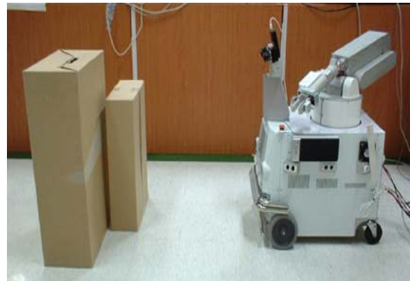
Fig. 1. Home Service Robot (Hombot) equipped with a stereo camera and a laser slit generator
