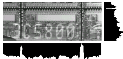
Fig. 6 Histogram profile of wafer ID image
