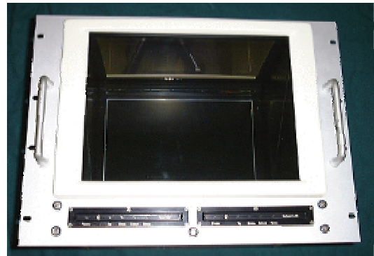
Fig.13 Polarization type stereo display with TFT-LCD
