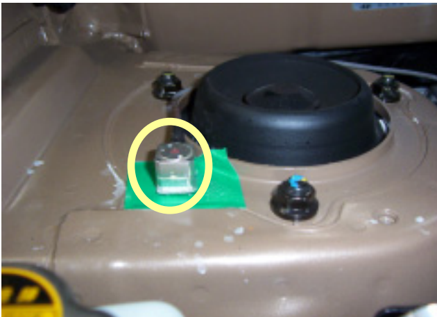
Fig. 4-2 Sensor installation: Accelerometer
