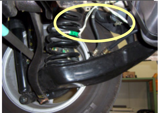
Fig. 4-3 Sensor installation: Strain gage
