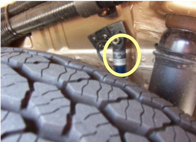
Fig. 4-1 Sensor installation: Potentiometer
