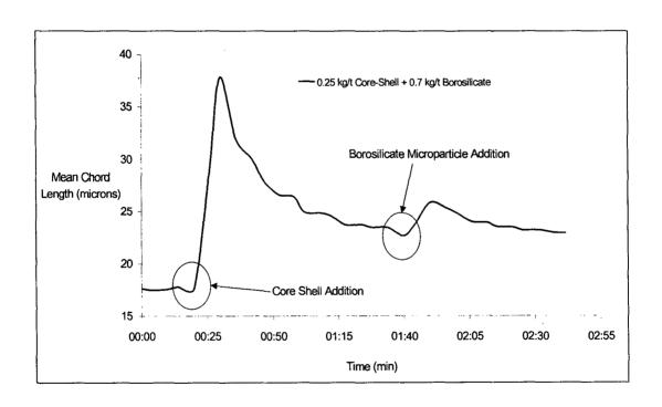
**Figure 8:** Comparison of the *Change in Mean Chord Length* after addition of borosilicate microparticle for different flocculants added at 0.25 kg/T.
