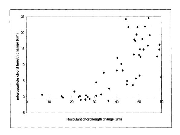
**Figure 7:** Re-flocculation of a LWC furnish by borosilicate microparticle added 80 seconds after flocculant addition.
