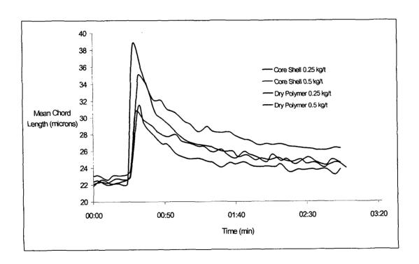
Figure 4: Comparison of Mean Chord Length data obtained after addition of Core Shell only, and a program consisting of a combination of dry polymer plus bentonite. Bentonite was added 5 seconds after the dry polymer.
