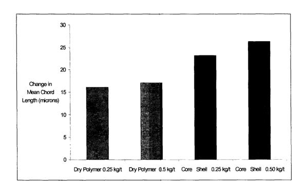
Figure 3: Comparison of Mean Chord Length data obtained after addition of Core Shell or dry polymer to an acid LWC furnish.
