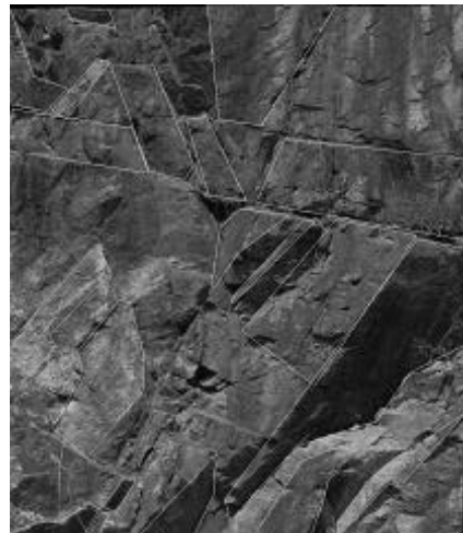
Fig. 5. Discontinuous plan of rock slope using automatic and manual linear extraction..
