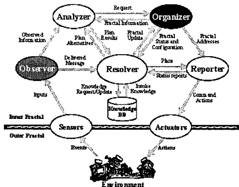
Figure 2. Functional modules and relationships of a BFU in the FrMS
