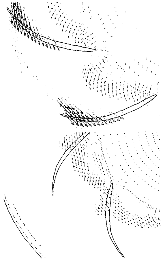
Fig. 7 Plots of meridional velocity vectors between sequence blades for backward blades blower (upper) and forward one
