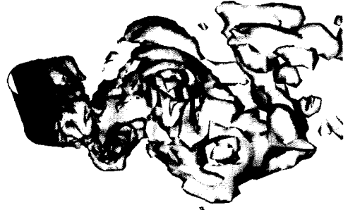
Fig. 10 Isosurface of instantaneous vorticity magnitude in the flow over a circular cylinder at Re=3,900
