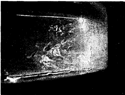
Fig. 8 Visualization of Streak lines captured by the laser sheet in rz-plane of DN type inflow device
