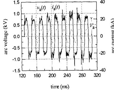
Fig. 1. Real arc voltage and current waveforms.
