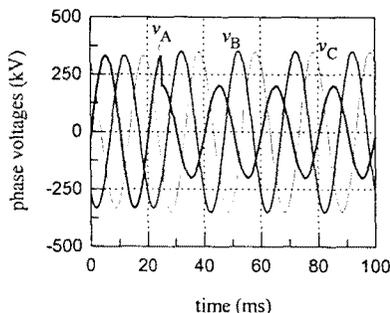
Fig. 9. Distorted input voltages generated by EMTP.
