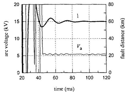
Fig. 11. Calculated fault distance and arc voltage amplitude.
