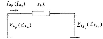
Fig. 5. Positive and negative sequence line equivalent circuit.
