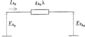
Fig. 6. Zero sequence line equivalent circuit.
