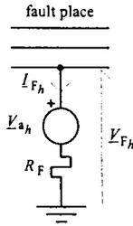
Fig. 3. Fault model given in spectral domain for  $h$ -th harmonic.
