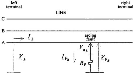
Fig. 4. Single-phase to ground arcing fault on three phase line.
