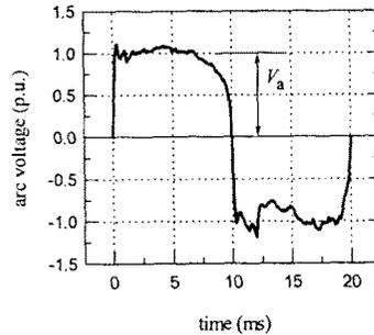
Fig. 2. Typical accepted arc voltage wave shape.
