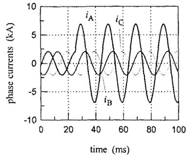
Fig. 10. Distorted input currents generated by EMTP.
