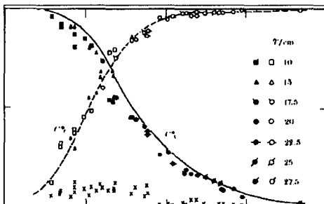
Fig. 1. Reflection and transmission coefficients for vertical thin plate. Full symbols are for transmission; hollow symbols are for reflection; the crosses are for energy dissipation (from Stiasnic et al., 1984).
