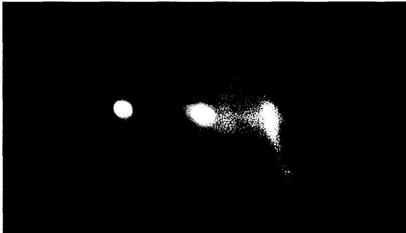
Fig 3. Photograph of fifth (213 nm), fourth (266 nm) and second (532 nm) harmonic beams separated by a prism (from left to right). Most of the second harmonic beams were blocked.
