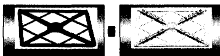
Figure 1. Take-up plate with fixed needle type (좌) Take-up plate with moving needle type (우)
