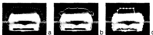
Figure 7. The results of infrared images containing vehicle, (a) input image and initial contour, (b) proposed method. (c) snake algorithm
