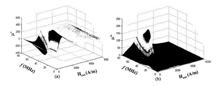
**Fig. 1.** The real  $[\mu]$ , in (a)] and imaginary  $[\mu]$ , in (b)] parts of magnetic permeability versus magnetic field  $H_{ext}$  and frequency f.
