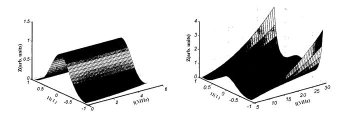
The magneto-impedance changes as a function of magnetic field at various frequencies (the left to right) up to 30 MHz.
