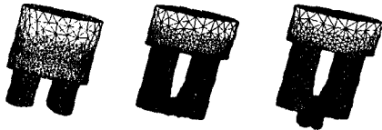
(A) Dividing (B) Welding (C) Forming Fig. 4 Each stage of a porthole die extrusion
