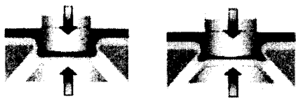
Fig. 2 2-step form-joining process
