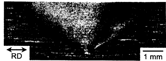
Fig. 3 Typical optical macrograph of cross-section perpendicular to the tool trajectory direction of the friction stir processed specimen
