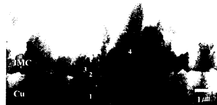
Fig. 2 STEM micrograph of a Sn-Cu-Ni/Cu interface aged at 120°C for 6days.
