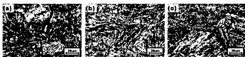
Fig 3. Microstructures of weld metal and quenched specimen (a) 4m/min (Hv=503), (b) 7m/min (Hv=505) and (c) Water quenched (Hv=505)
