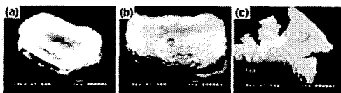
Fig. 7 SEM microstructures of oxidized NbC on tilt 45°
