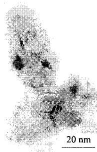
Fig. 1 HRTEM of composite \gamma\text{-Fe}_4\text{N}/\alpha\text{-Fe} nanoparticles
