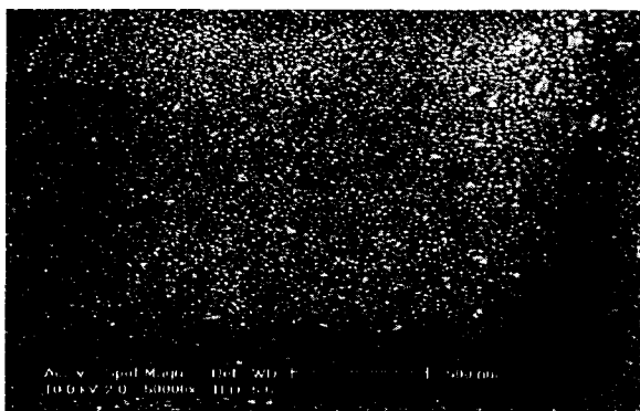
Fig. 4. SEM micrograph of the surface of 35nm thickness Y_2O_3 film, which were grown at 700^\circ C and 2 \times 10^{-5} Torr. This figure showed no cracks.
