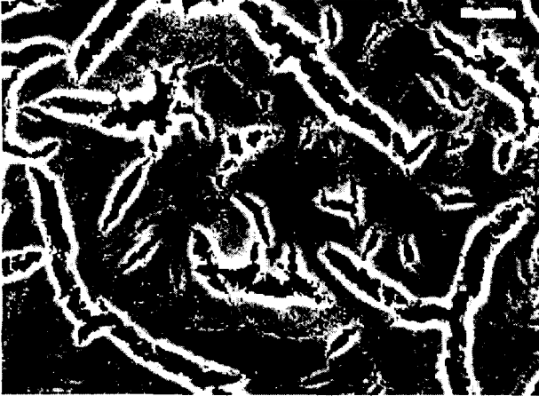
Fig. 5. SEM image of Y_2O_3 in acetic acid coated Ni tape. (Scale bar indicate 1\mu m .)
