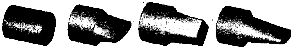
Fig.6 passes of roll forging of blank
