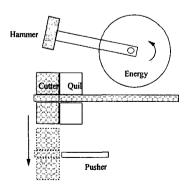
A hammer unit stores energy in the form of kinetic, potential or pressure, and releases it by impacting a cutter unit. The hammer must have enough mass and travel over a target shear speed at its impact.
