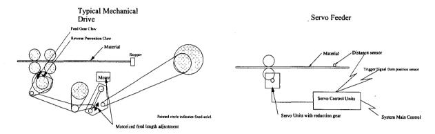
Simpler structure gives a cost advantage over mechanical one. The adjustment of cut-off is straightforward. Key components of this mechanism are a servomotor and distance sensor.
