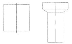
Cropping → Annealing → Surface treatment → Cold Extrusion-→ Sub-critical Annealing → machining → Carburizing → Polish
