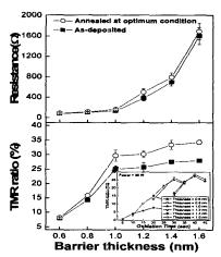
Fig. 1 TMR ratio and resistance variations of the MTJ with ZrAl-oxide barrier as a function of barreir thickness. Samples were annealed at optimum temperatures as a function of barrier thickness for 10 min.
