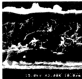
Figure 2. Cross sectional SEM image of the FS 1000 reinforced composite membrane.
