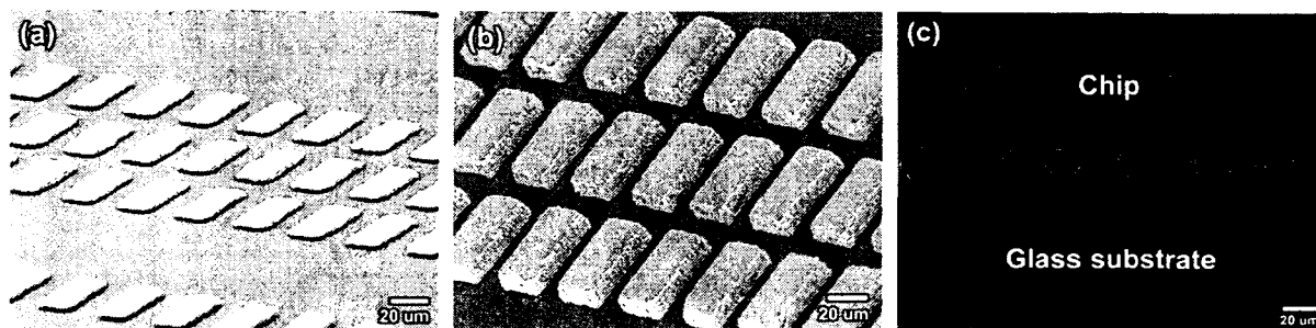
Fig. 5. SEM images showing (a) the metal pads, (b) the Sn solder bumps, and (c) 40 \mu\text{m} pitch In/Sn solder joints.
