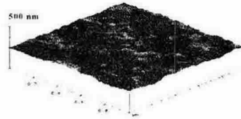
(b) KOH 1 min \rightarrow Ar + treatment 20 min, Ra=0.38
