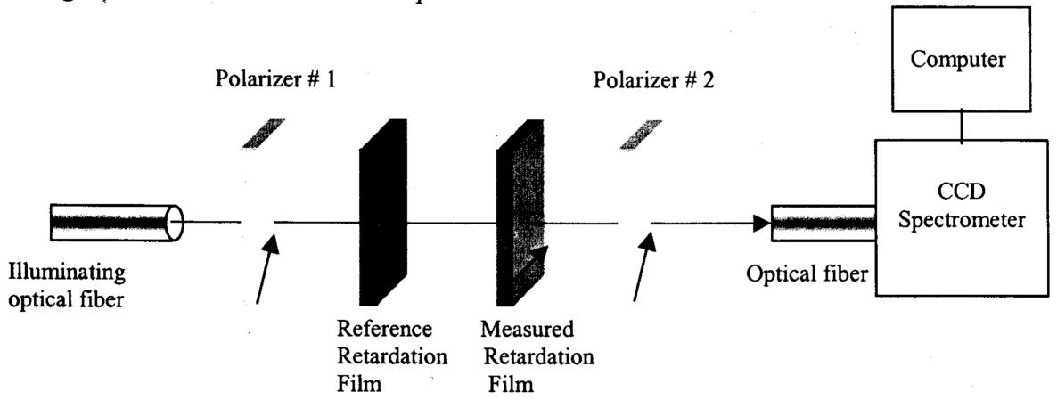
Fig. 1 Retardation measurement scheme (films axes are indicated by arrows)
