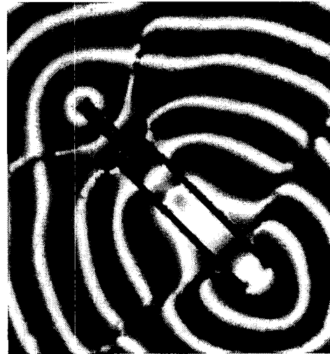
Fig. 8 Acoustic pressure radiation pattern of Fig. 7
