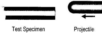
Figure 8 The eccentric impact of the projectile to generate the longitudinal and flexural waves simultaneously
