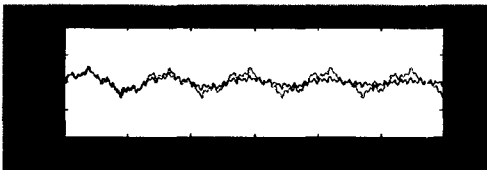
Fig. 11 Response of uncontrolled and controlled beam for arbitrary disturbances (actuator position = l/10 )
